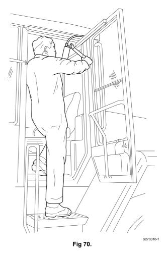
When you grease the cab door hinges, open the door and stand as shown.
