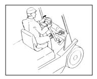
Release brake pedal and depress the accelerator pedal to start the truck.
