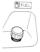
The fuel reservoir cap is located at the rear left side of the truck body. To open, turn it counterclockwise.
