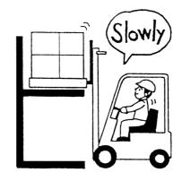
Operate hydraulic control levers slowly when loading and unloading. There is a danger of falling load or overturning the truck when operating the levers suddenly at high height position of forks.
