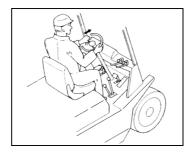
Gradually release the clutch pedal while depressing the accelerator pedal to start the truck.
